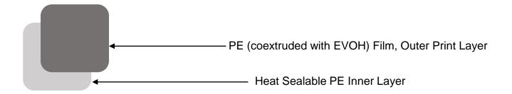
The #4 Recyclable structure is a mono-material constructed out of two layers of Low Density Polyethylene (PE). It contains less than 5% of a copolymer known as EVOH, which provides excellent oxygen and moisture barrier properties. PE zipper optional on preformed pouches. Mono-material means that it can be used to create sustainable flexible packaging options that comply with international recyclability guidelines.
